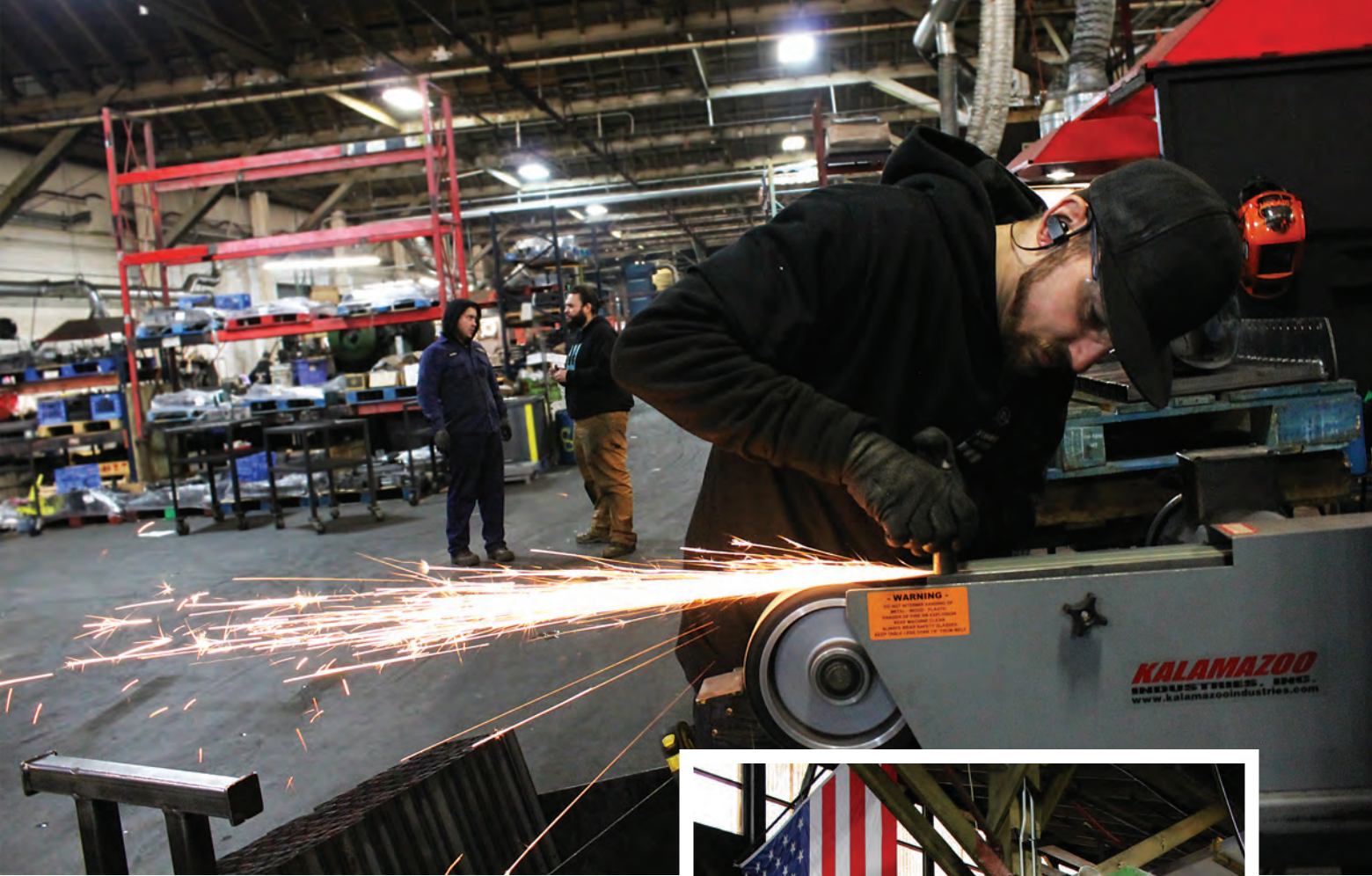
Torklift's Spencer Grant grinds down the edges of a piece of metal that will be welded to an attachment plate to create the main portion of the company's All Terrain Landing Gear.
