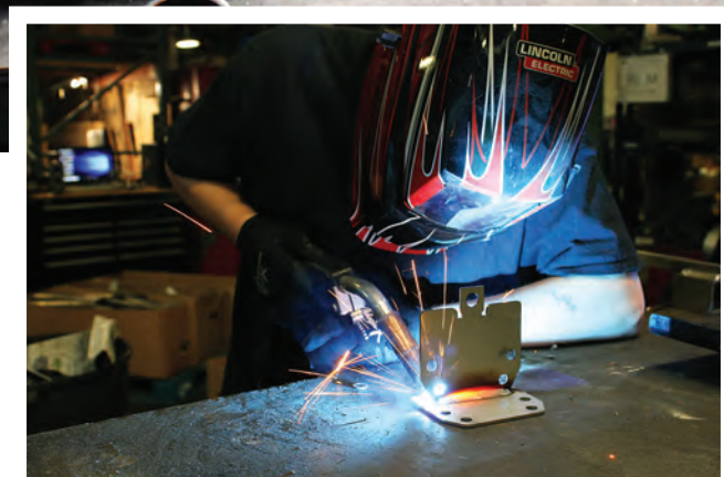
Torklift's Arturo Macdenado (above) welds the final pieces of a receiver onto a hitch before attaching it to the crossbar. Torklift's Austin Bryan (right) welds together two parts before bending them into Torklift Derringer Handles for turnbuckles.
