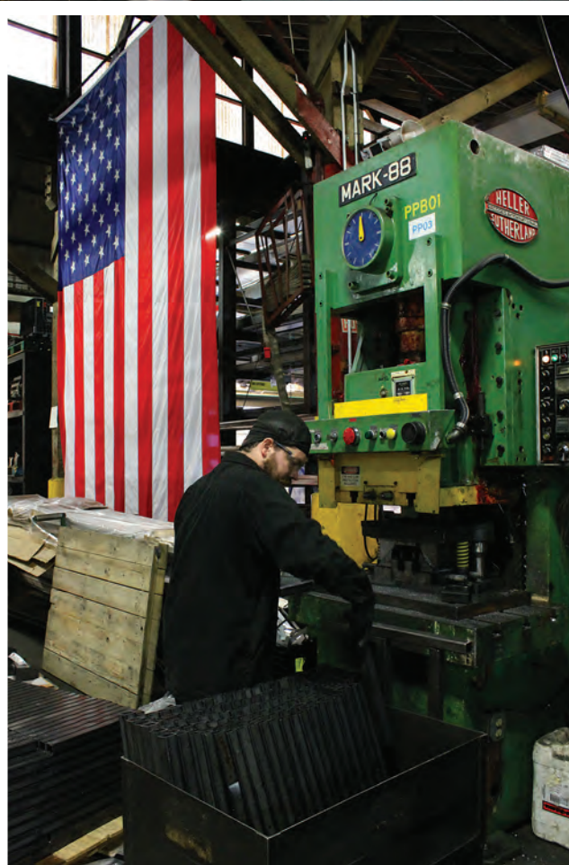
Torklift's Wes Love operates a machine that punches holes into metal pieces that will be turned into the All Terrain Landing Gear feet. Each piece is meticulously punched to make sure quality is the same on all pieces.
