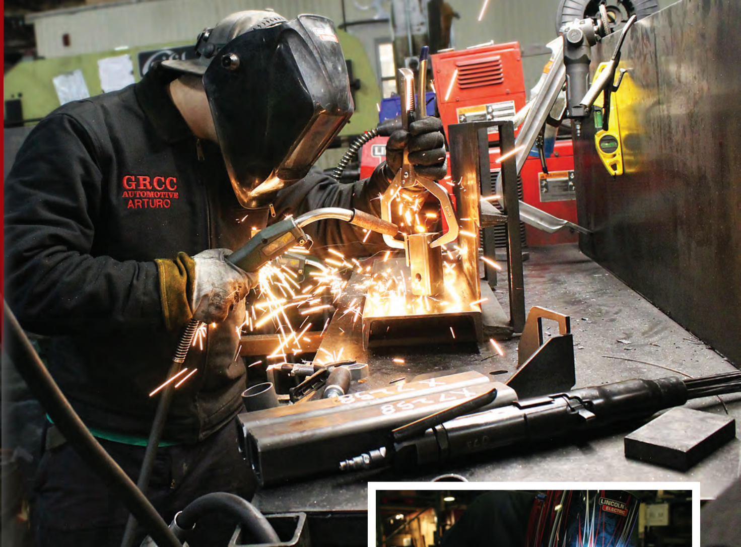
Torklift's Arturo Macdenado (above) welds the final pieces of a receiver onto a hitch before attaching it to the crossbar. Torklift's Austin Bryan (right) welds together two parts before bending them into Torklift Derringer Handles for turnbuckles.
